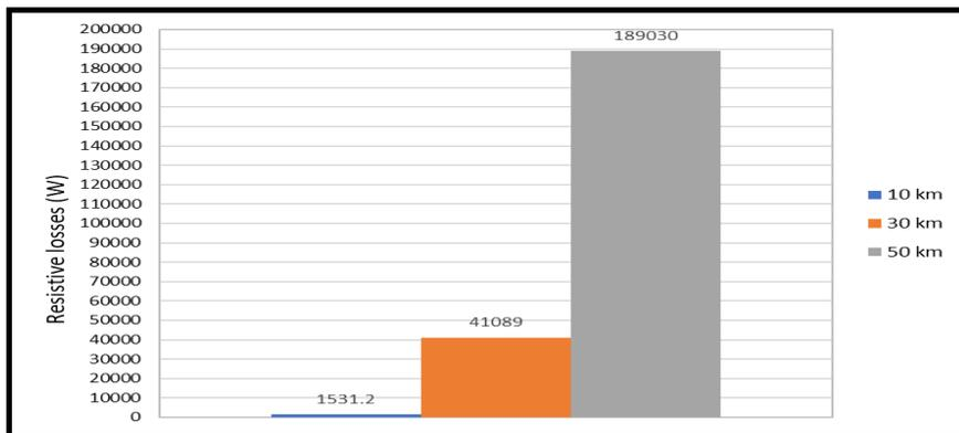
Fig. 19: Corresponding losses per screen (W) for single-point bonding
