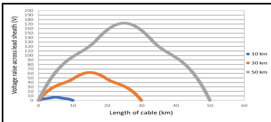
Fig. 18. Voltage raises across lead sheath (V) for cross bonding
