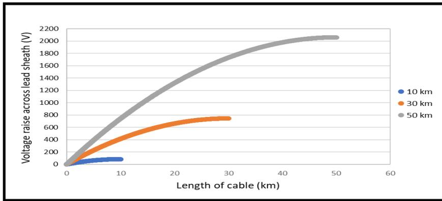
Fig. 16. Voltage raises across lead sheath (V) for single-point bonding
