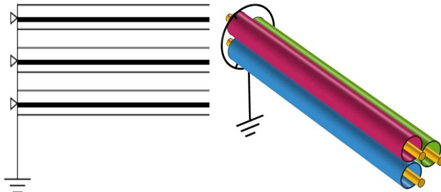
Fig. 1. Arrangement for single-point bonding
