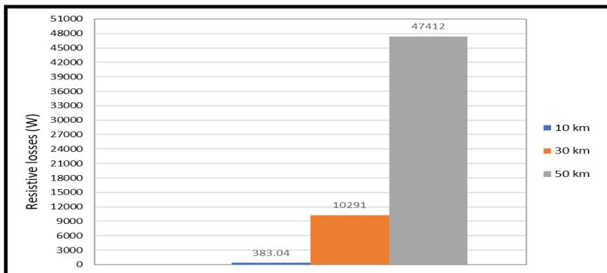
Fig. 20: Corresponding losses per screen (W) for solid bonding
