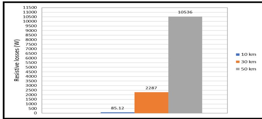
Fig. 21: Corresponding losses per screen (W) for cross bonding
