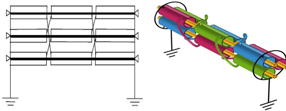
Fig. 3. Arrangement for cross bonding
