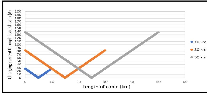
Fig. 14. Charging current through lead sheath (A) for solid bonding
