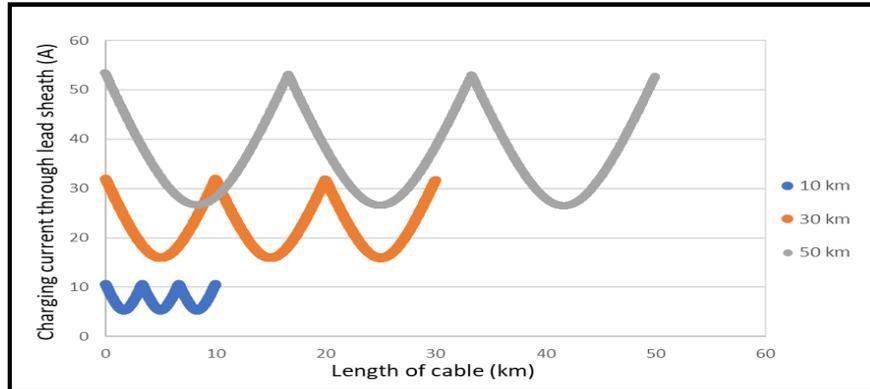
Fig. 15. Charging current through lead sheath (A) for cross bonding
