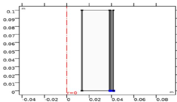
Fig. 10. 2D Geometry of single-point bonding method
