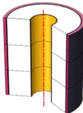
Fig. 8. The cable's 2D axisymmetric geometry
