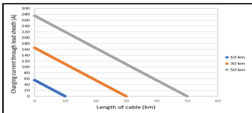
Fig. 13. Charging current through lead sheath (A) for single-point bonding
