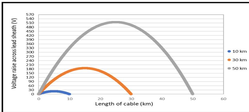
Fig. 17. Voltage raises across lead sheath (V) for solid bonding
