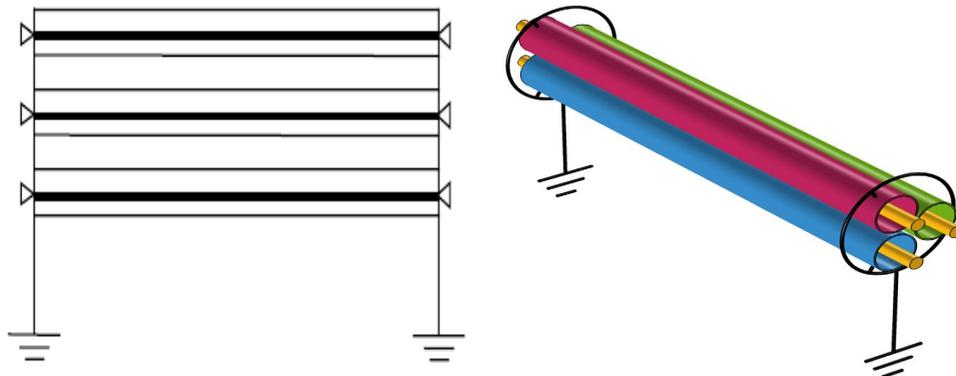
Fig. 2. Arrangement for solid bonding
