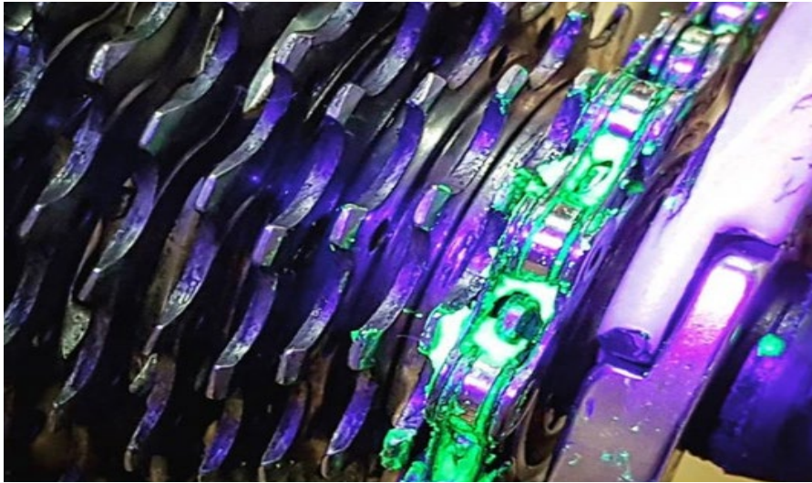
Fig. 3. UV dye injected into lubricant for better observation
