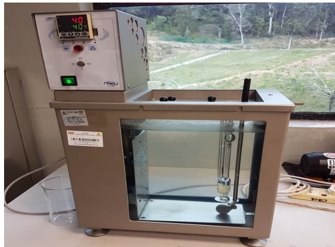
Fig. 2. Calibrated glass capillary viscometer to perform kinematic viscosity of the lubricant
