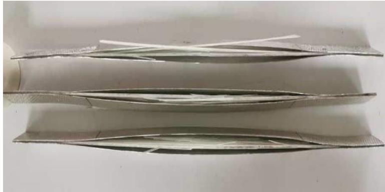
Figure 8. Plastic deformation and delamination of Al 2024-T3 layer post failure
