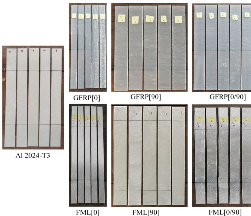
Figure 2. Specimens of aluminium alloy 2024-T3, GFRP composite and FML
