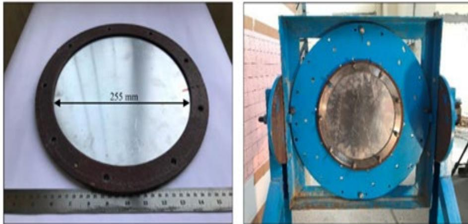
Figure 1. The circular target plate fully fixed around its outer perimeter leaving a 255 mm in diameter central exposed area [16]
