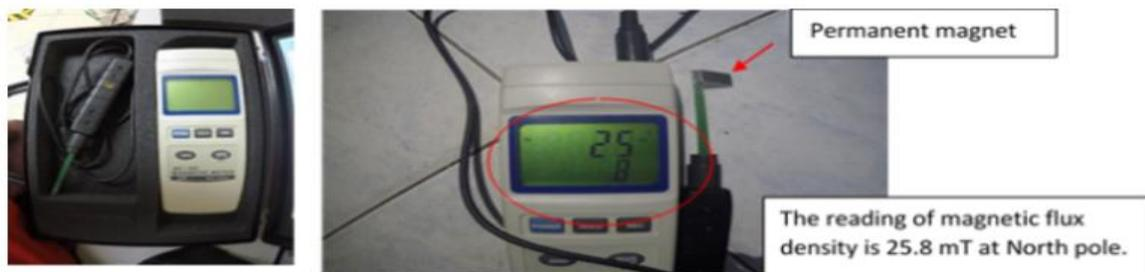
Figure 14. Magnetic meter reading
