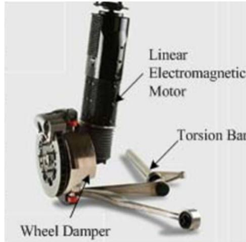
Figure 9. Electromagnetic suspension developed by Bose [20]
