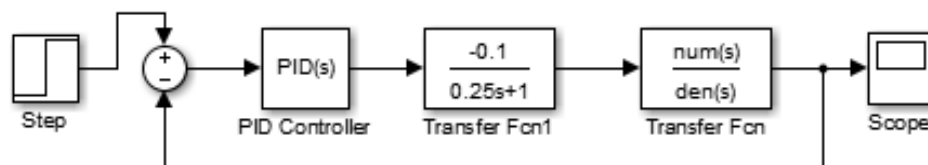
Figure 18. Simulink diagram for PID controller for P15035 Aircraft
