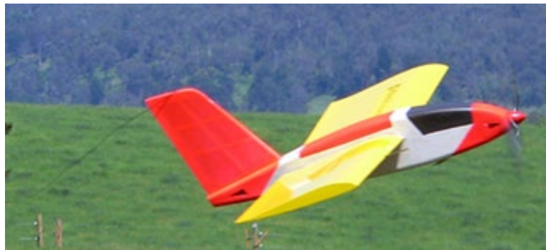
Figure 11. The P15035 Aircraft with single motor and elevons
