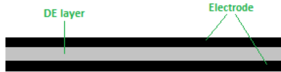
Figure 2. Dielectric elastomer generator (DEG) illustration
